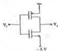
The threshold voltage for each transistor in the figure shown above is 20 V. What are the values of V<sub>i</sub> for this circuit to work as an inverter?
