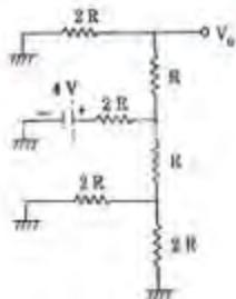
What is the output voltage 'V<sub>o</sub>' of the R-2R decoder ladder network?
