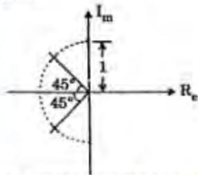
A diaphragm type pressure sensor has two poles as shown in the figure above. The zeros are at infinity. What is its steady state deformation for a unit step input pressure?
