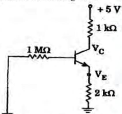
What is voltage difference between collector and emitter ( $V_{CE}$ ) in the above circuit?
