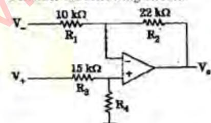
What is the value of  $R_4$  in the above circuit, if the voltage  $V_-$  and  $V_+$  are to be amplified by the same amplification factor?
