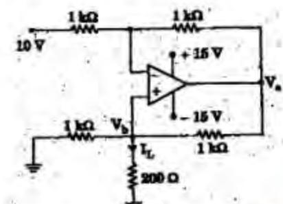
What is the load current  $I_L$  in the above circuit?
