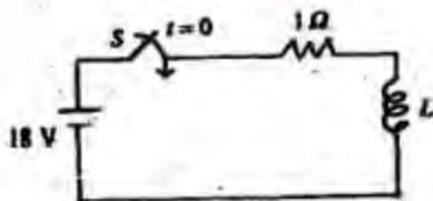
In the above circuit, S was initially open. At time  $t = 0$ , S is closed. When the current through the inductor is 6 A, the rate of change of current through the resistor is 6 A/s. The value of the inductor would be
