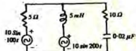
Which one of the following theorems can be conveniently used to calculate the power consumed by the  $10 \Omega$  resistor in the network shown in the above figure?
