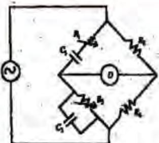
The Wein bridge circuit shown in the above figure can be used as a frequency measuring device, provided
