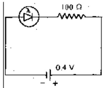
A photodiode is connected as shown in figure. When the device is illuminated with light of intensity  $100 \text{ lm/cm}^2$ , a current of  $1.8 \text{ mA}$  flows in the circuit. Calculate the resistance offered by the photodiode. If the illumination is doubled, what happens to the resistance value?
