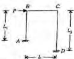
The shear equation for the portal frame shown in the above figure will be
