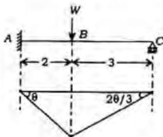
If a uniform beam shown in the figure above has the plastic moment capacity  $M_p$  for span AB and 0.9  $M_p$  for span BC, what is the correct virtual work equation?
