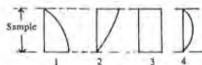
Excess pore pressure distribution within the thickness of a soil sample tested in oedometry sometime after loading is shown in the above figures labeled 1, 2, 3 and 4. Which one of these figures, refers to a situation where the operator forgot to put
