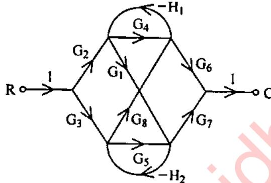
Obtain  $\frac{C}{R}$  from the signal flow graph shown in the above figure using Mason's Gain Formula. 5
