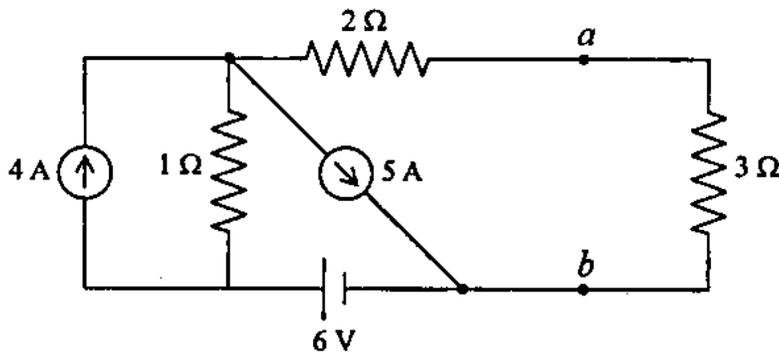
For the above circuit, determine the voltage across 3 ohm resistor applying Thevenin's theorem. State the maximum power theorem for an ac circuit. 12
