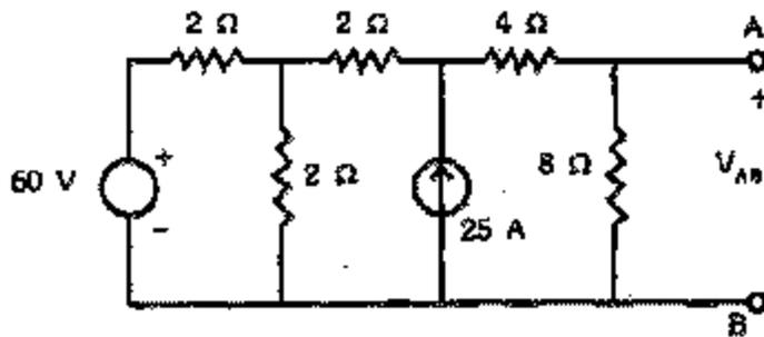
Find  $V_{AB}$  for the circuit shown above using source transformation.
