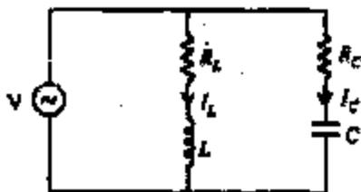
For the circuit shown above, draw the phasor diagram. Derive the condition for the two branch currents,  $I_L$  and  $I_C$ , to be in quadrature.
