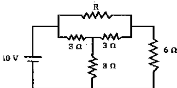
Determine the value of  $R$  shown in the above figure such that the  $6\ \Omega$ -resistor consumes the maximum power.
