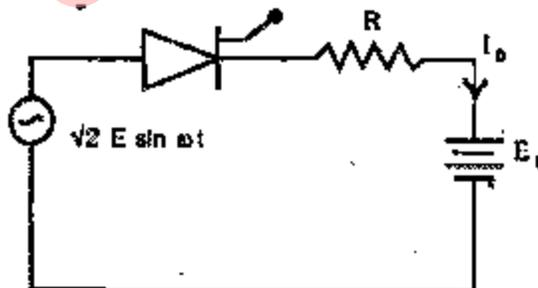
Derive an expression for the average charging current in terms of source voltage  $E$ , back e.m.f. and resistance  $R$ . The SCR is fired continuously. If  $E = 220 \text{ V}$  (r.m.s.),  $E_b = 100 \text{ (DC)}$  and  $R = 10 \text{ ohms}$ , calculate —
