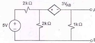
Q.59 For the circuit given above, the Thevenin's resistance across the terminals A and B is
