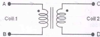
The figure above shows coils 1 and 2, with dot markings as shown, having 4000 and 6000 turns respectively. Both the coils have a rated current of 25 A. Coil 1 is excited with single phase, 400 V, 50 Hz supply.
