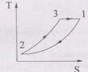
Q.75 If the specific heats of the working fluid are constant and the value of specific heat ratio  $\gamma$  is 1.4, the thermal efficiency (%) of the cycle is
