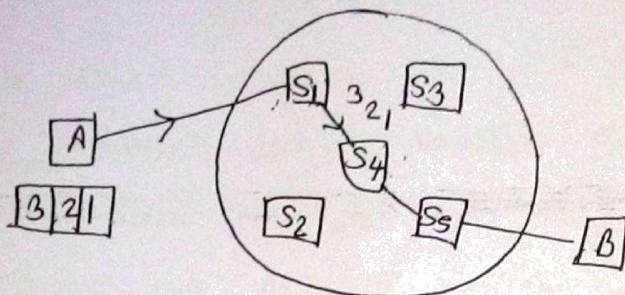
Here first each switch will check & establish the connection. Then that connection will get freeze. Now after connection is fixed, message is divided into different packets known as datagram. These message switch  $S_1$  will transfer all the packets after some duration to the next switch. Now here next intermediate switch  $S_4$  will send the packets to next one.
