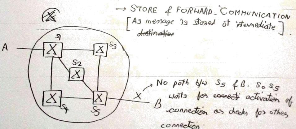
→ Not reliable way of switching as here no acknowledgement is sent to sender whether message is received or not.
