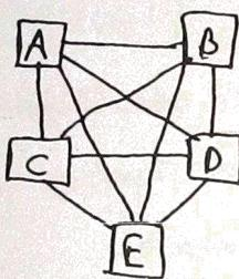
No. of wires required to establish the mesh topology are
