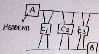
→ If  $C_i$  is connected upstream then bus A (upper bus) is primary bus & lower bus is secondary bus.
