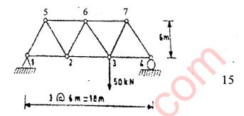
9. Analyze the truss as shown in figure by method of tension coefficients and determine the forces in the members AB, AE and BE.
