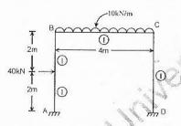
9. Analyze the frame shown below by Cantilever Method.
