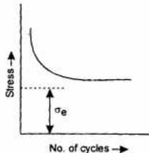
**Size Factor :** If the size of standard specimen will increase, then the endurance limit of the material will decrease. This is due the fact that a longer specimen will have more defects than a smaller one.
