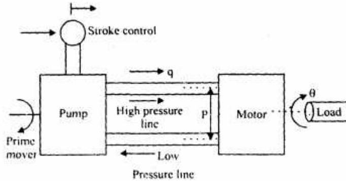
The transfer function of the system is given by
