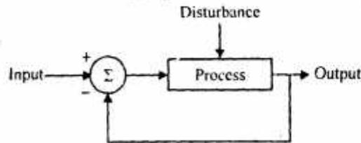
Here it contains feedback so that whatever be the output it's feeded back to the next input hence error is measured.
