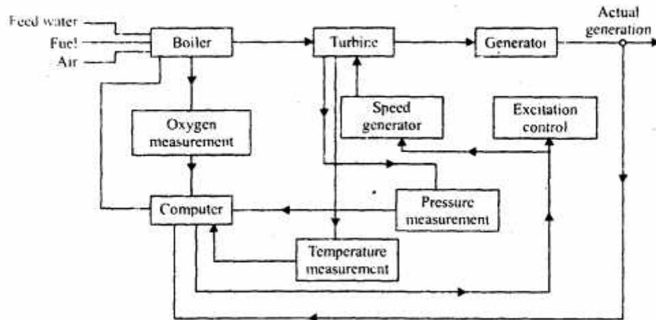
The boiler control system is shown in above figure, it has :
