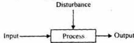
Input and by process we get output respectively. Here no feedback is provided so open loop.
