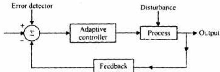
Here the adaptive controller is shown so that we can use any alternative controller i.e., proportional or integral or derivative or their combinations are used.
