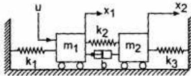
Ans. The equivalent mechanical system will be as shown :
