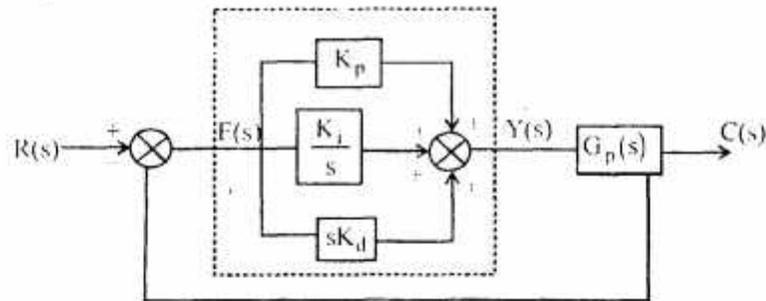
In the diagram, the PDI type hydraulic controller is shown inside the dotted lines.
