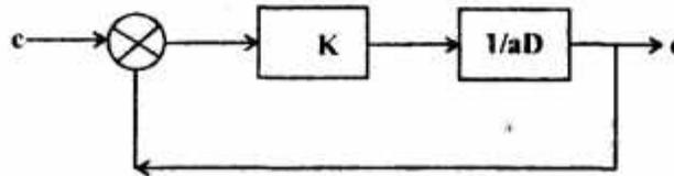
**Ans.** The open loop transfer function of the given first order system is given by :
