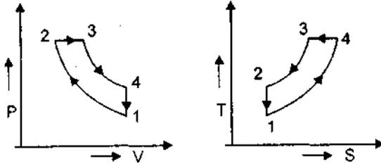
$$T_1 = 300 \text{ K}, P_1 = 1.01 \text{ bar } r = 20, \rho = 2 \quad r = \left( \frac{V_1}{V_2} \right)$$
