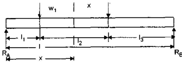
Consider a simply supported beam AB having two concentrated load  $W_1$  and  $W_2$  as shown in figure.
