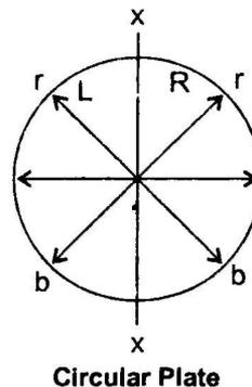
When a beam of white light, rendered plane polarised by the polarising Nicol, is incident normally in the bi-quartz plates, it rotates the different wavelengths of white light to different extents, thus, rotatory dispersion occurs in each plane.
