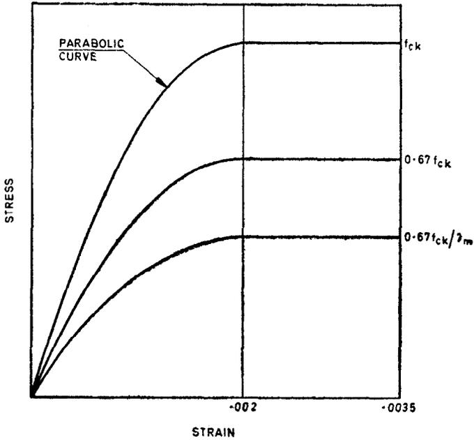
FIG. 3 STRESS STRAIN CURVE FOR CONCRETE
