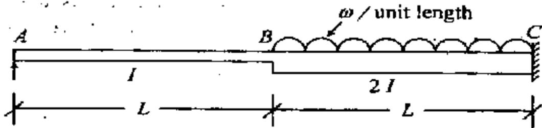
A stepped beam  $ABC$ , simply supported at  $A$  and fixed at  $C$  as shown in the above figure carries a uniformly distributed load of intensity ' $\omega$ ' per unit length over  $BC$ . Determine the vertical reaction at  $A$  using moment area or energy method. 20
