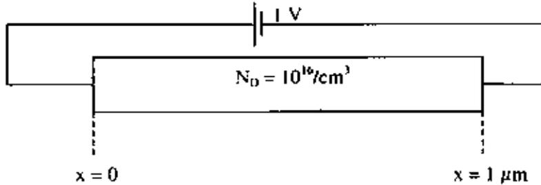
Q.52 The magnitude of the electric field at  $x = 0.5 \mu\text{m}$  is
